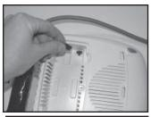
3. Connect the battery pack cable to the unit's battery connector in the bottom of the battery recess.
