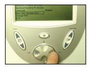
Press the Display button to accept the highlighted selection.
