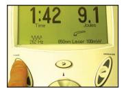
3. Press the TIME button and raise or lower treatment time using the up and down arrows.
