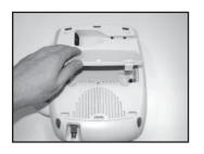
2. Remove the battery access door and retain this cover.
