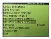
2. Press the Up Arrow or Down Arrow buttons to highlight the Restore Factory Protocols option.
