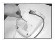
1. Locate the battery access door at the bottom of the unit and loosen the screw with a regular screwdriver.
