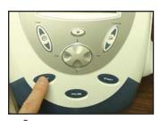
4. Press the DOSAGE button and raise or lower the unit's output using the up and down arrows.
