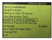
2. Press the Up Arrow or Down Arrow buttons to highlight the Restore Factory Settings option.
