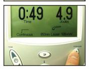
6. Press the DISPLAY (Enter) button to accept the highlighted selection.
