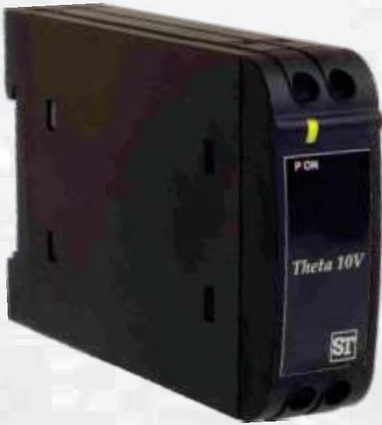
*Theta 10A / 10V* transducer converts a sinusoidal AC Current or AC Voltage into a load independent DC Current or a load independent DC Voltage proportional to the measured value.
