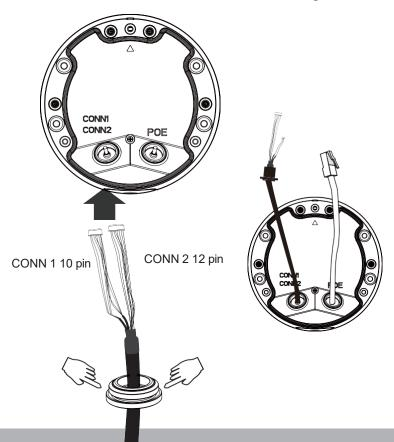
B-2. Connect the pin headers to the I/O extension module and that on the camera. Note the orientation of the pin headers with the positions of the tabs. Properly install the grommet as previously described.
