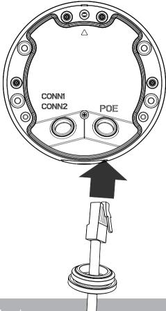
7. When installing the silicon grommet, make sure the cable is slightly pulled back to the outside. Do not leave the rim of the seal jammed in the inside of the seal.
