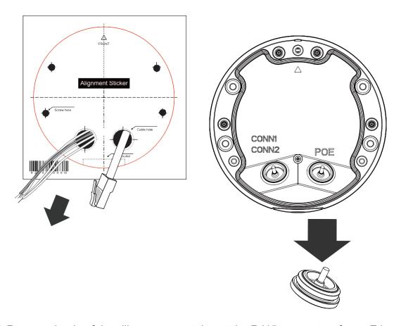
4. Remove the tip of the silicon grommet. Insert the RJ45 connector of your Ethernet cable into the penetration cap.
