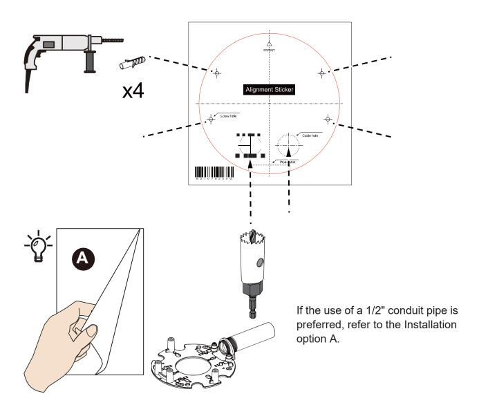
3. Route cables through the wall or ceiling, and remove the grommet from the base plate.
