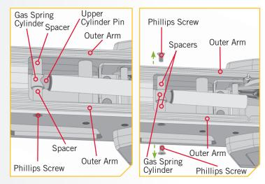
**NOTICE:** Use a #3 Philips screwdriver to remove the screws. They have a pre-applied thread locker. Not using the recommended tool can cause damage and prevent them from being removed.
