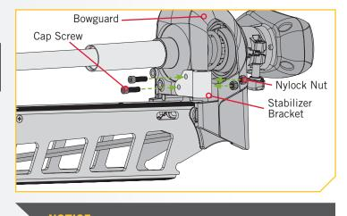
NOTICE: The two Lock Washers (Item #16) are not used when installing on the Fortrex.
