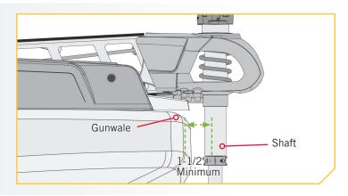
g. Once the Mount is in position, determine which bolt pattern to use. The bolt pattern selected will depend on the deck space available on your boat.
