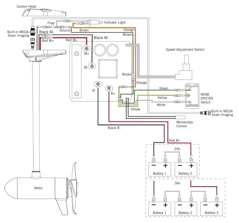
**NOTICE:** This is a multi-voltage diagram. Double-check your motor's voltage for proper connections. Over-Current Protection Devices are not shown in this illustration.
