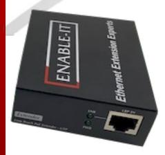
You can add additional 328ft (100m) onto the end of each 821 LAN output ports for a total distance of 2,306ft (702m) from device extension to device extension.
