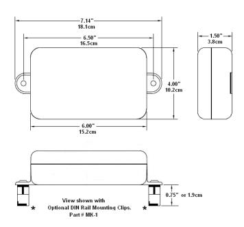
The D6000 series modules can be easily adapted to a DIN rail using the DGH MK-1 mounting kit shown in view above.
