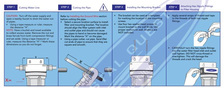
\*Measure to shoulder inside of fittings. Copper pipe butts against this shoulder.
