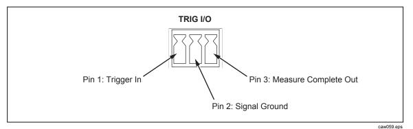
Figure 4-9. TRIG I/O Pin-out Description
