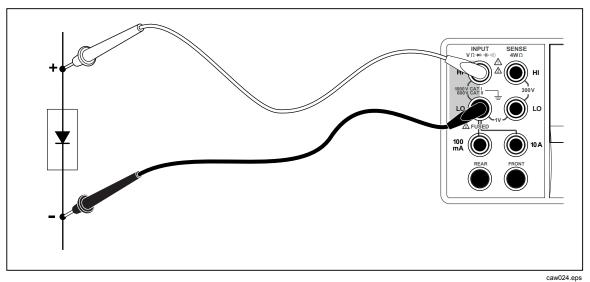
Figure 4-8. Diode Testing Connections
