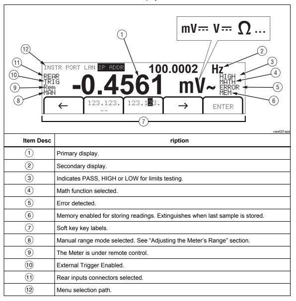
Measurement results occupy the first two rows of the display. The primary display consists of larger sized characters that comprise the  $6\frac{1}{2}$  digits (-1999999 to 1999999), plus a decimal point. In the example shown above, the primary display shows measurement results for an ac voltage measurement.
