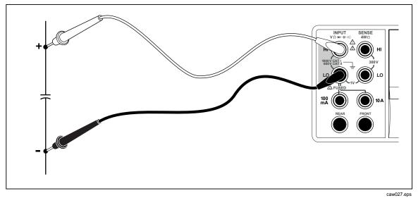
Figure 4-6. Measuring Capacitance
