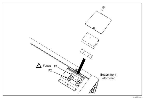
Figure 2-2. Replacing the Current Input Fuses
