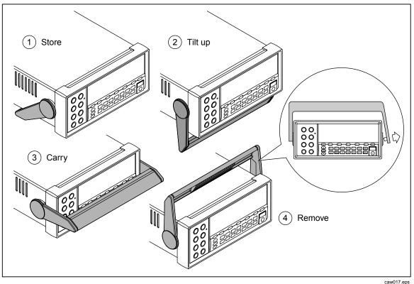
Figure 2-4. Bail Adjustment and Removal
