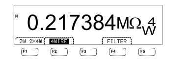
3. If not already highlighted as shown above, press the 4WIRE soft key to switch to a four-wire measurement.
