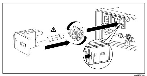
Figure 2-1. Replacing the Line Fuse
