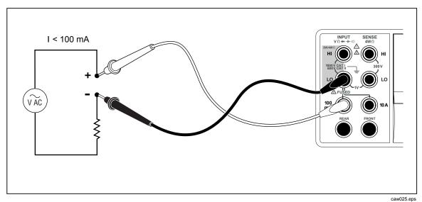
Figure 4-4. Input Connections for Current Measurements Below 120 mA
