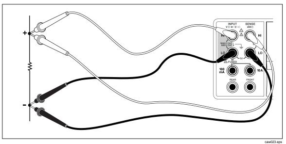
Figure 4-2. Input Connections for 4-Wire Resistance Measurements
