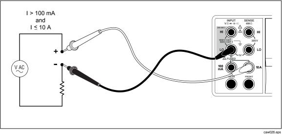
Figure 4-5. Input Connections for Current Measurements Above 120 mA
