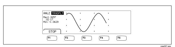
As shown in Figure 3-1, the display will start plotting the readings across the plot area, and the maximum, minimum, and elapsed time are displayed.
